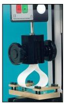
**Procedure:** An adhesive ribbon 25 mm wide and at least 175 mm long is attached to the clamp of a dynamometer. The loop is placed in contact with a stainless steel plate (or other material) in a contact area of 25 X 25 mm and is detached at a speed of 300 mm/min.
